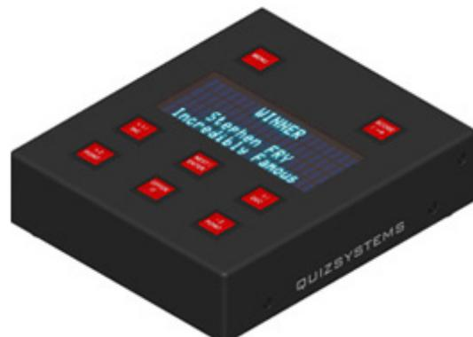
A QuizMasterDisplay (shown on the left above) provides 'who buzzed first' information, together with running team scores to anyone that requires it, while a QuizMaster (shown on the right), is a fully featured system control box (normally positioned backstage and operated by one of our technicians).
