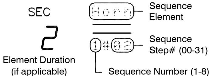
In the above, you can see that step#02 in sequence#1 is currently a two second horn (we've lifted this from the earlier '541L' sequence example).
