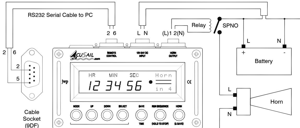
As an alternative to undertaking this wiring yourself, a high-powered (32A) relay unit, providing all of the necessary connectivity shown in this diagram (excluding the RS232 PC connection), is available. This accessory is supplied in a similar box to **AcuSail**, is splash proof (to IP64) and bolts underneath the main **AcuSail** unit.
