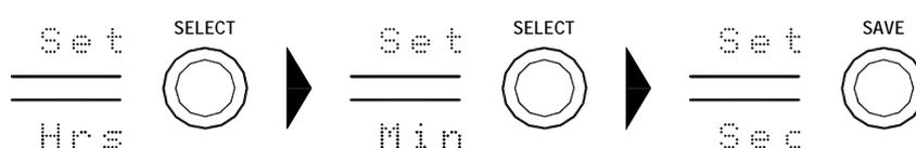
If you are subsequently unhappy with how well the **AcuSail** time display matches the real time (say for example because you pressed the *Save* button late), simply hold the *Save* button for at least three seconds, which will cancel the clock and allow you to repeat the setting procedure. Note that this function is automatically disabled once you have run any sequence.
