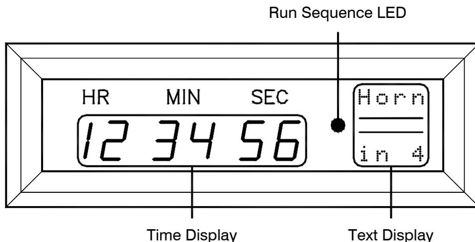
Times are always shown in the *Time Display* area, although occasionally (whilst setting the date for example), this area is used for other functions.
